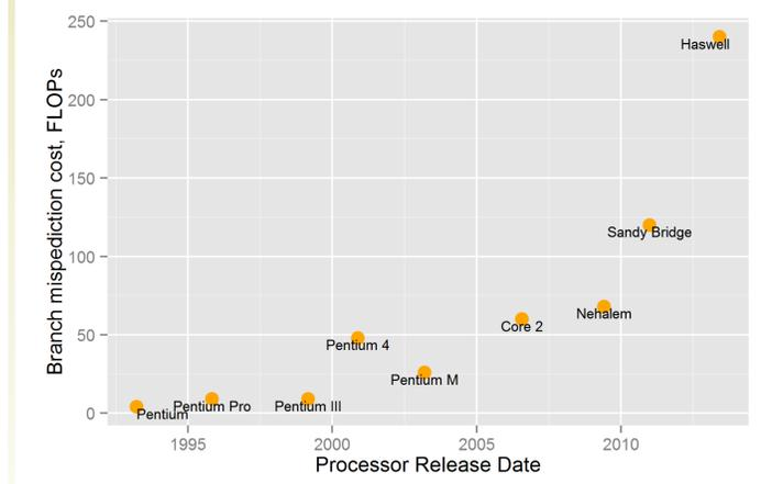
For this reason we avoid piecewise approximations and use branches only to detect special cases (such as NaN or infinite input), which do not normally happen and thus are predictable.
