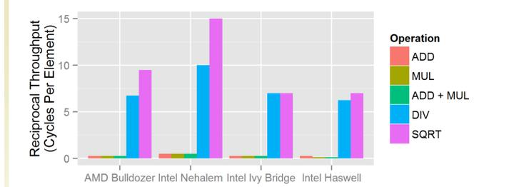
While most processors can issue multiplication and addition each cycle, division and square root are not pipelined, and have much lower throughput. We suggest that these operations should be avoided in favor of polynomial approximations and Newton-Raphson iterations.
