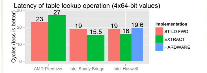
The total latency of such table lookup operations is too high to hide it with software pipelining or out-of-order execution. Although the recent Intel Haswell microarchitecture provides a hardware GATHER instruction, it does not reduce the latency.
